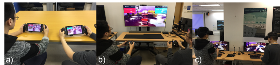
Figure 1: Examples of paired users during the experiment: (a) small display setup: two participants each using one small tablet display, (b) large display setup: two participants playing the game via a shared large display, and (c) VR HMDs setup: two participants playing the game while wearing the VR HMDs.
