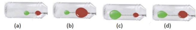
Figure 2: Four configurations of the center of gravity: (a) no balloon is filled (Empty); (b) the back balloon is filled (Back); (c) the front balloon is filled (Front); (d) both balloons are half-filled (Both). The summed weight is 50 g.
