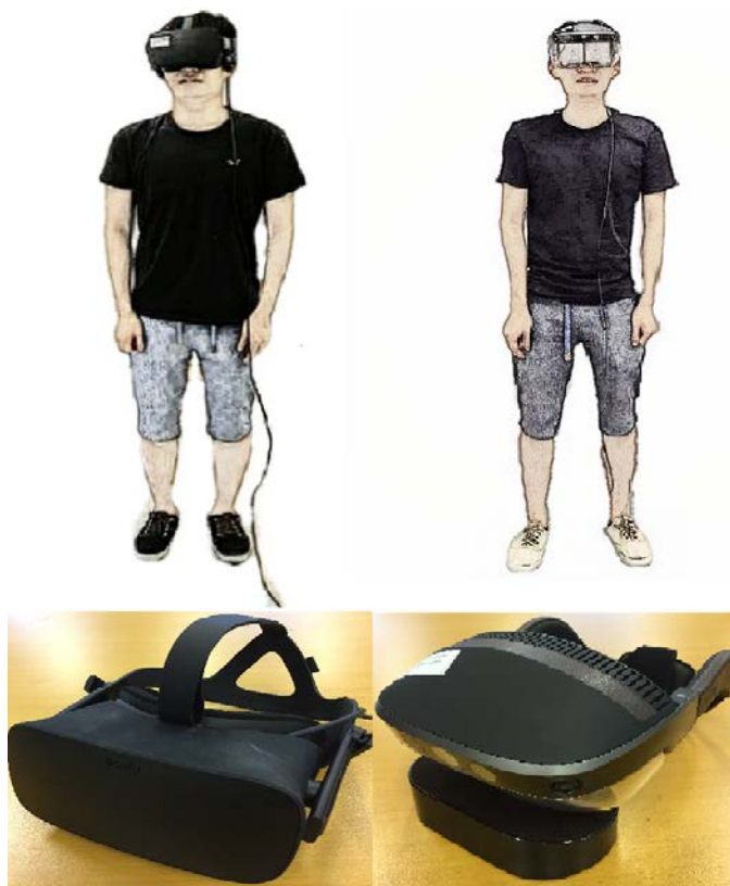
Fig. 1. Experiment setup with a user wearing the Oculus RIFT CV1 (left) and the user wearing the Meta 2 (right).
